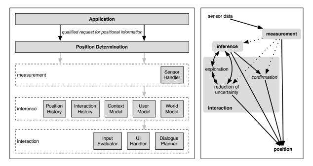
Figure 1: Example positioning architecture implementing the QoS model (left), and processes involved in determining the user's position: measurement, inference and interaction (right).
