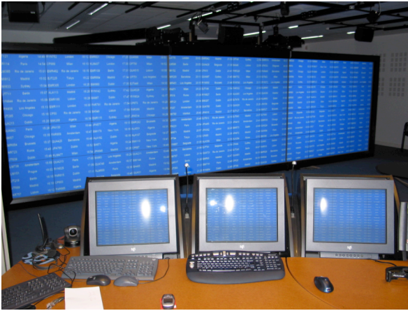
Fig. 6. Display setup, using a 3-screen CAVE in a “wall” arrangement.
